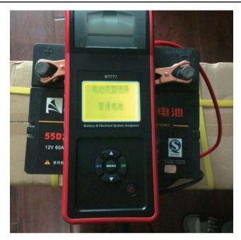
As the minimum width of the current clamp jaw is only 28mm, choose the connection cable or connection pole with diameter less than 28mm to test. Otherwise, the current clamp jaw cannot close completely.
