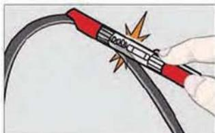
With the engine running, simply place the grooved end over the spark plug wire and the high intensity bulb will flash indicating spark
